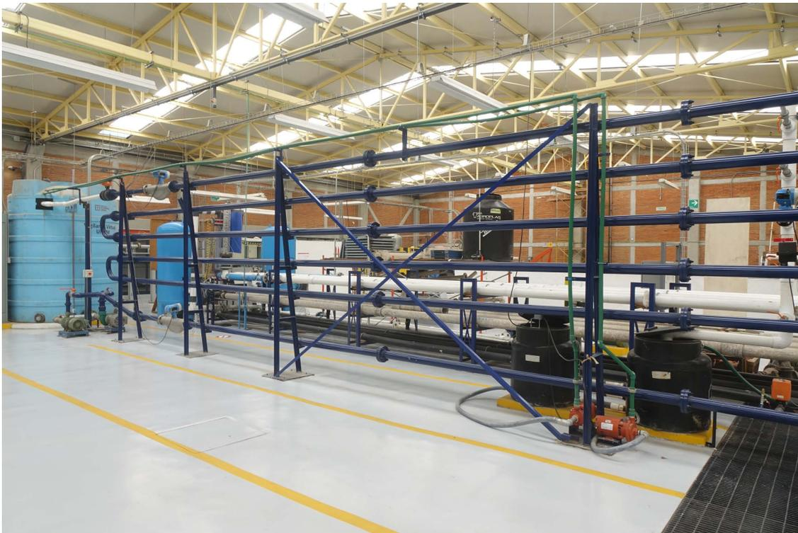
Fig. 7.1: Partial view of the facility. Pipeline in blue to the right and hydraulic pumps, instruments and water reservoir to the left
