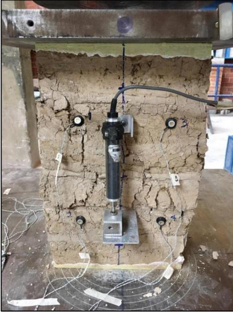
**Figura 6.37** Pila observa falla (Lado A)
