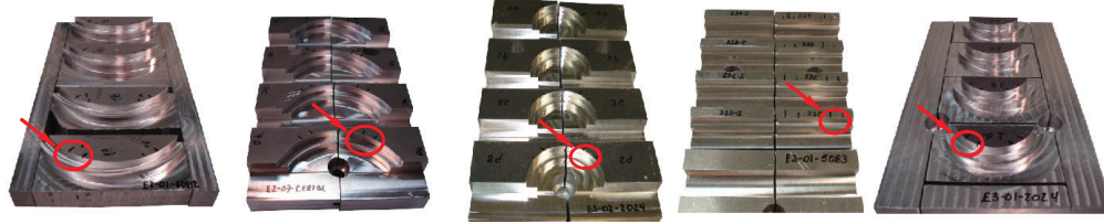
Fig. 2.4: Identification of the area for measuring the Ra in the specimens
